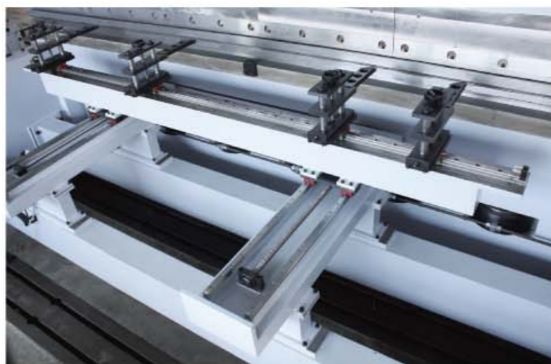
X-R 重型后挡料(选配) X-R heavy type backgauge structure
